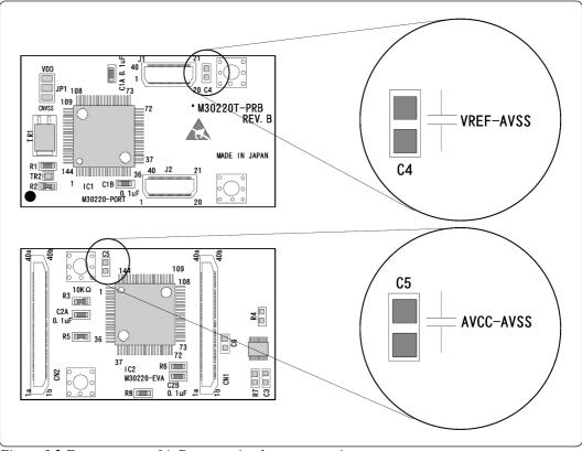
Figure 3.2 Foot patterns of A-D conversion bypass capacitor
